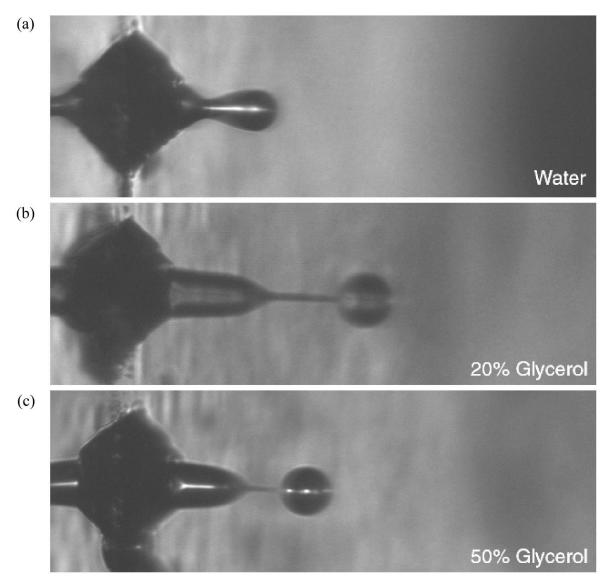
Fig. 4. Droplet formation versus increasing viscosity (a) water (b) 20% glycerol in water, (c) 50% glycerol in water.
