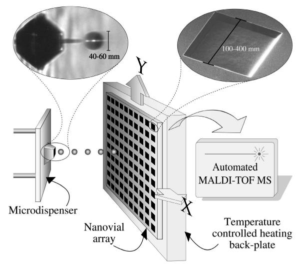
Fig. 10. Schematic drawing of the spot-on-a-chip amplification platform.
