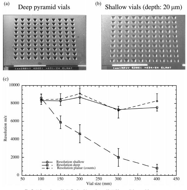
Fig. 7. (a) Inverted pyramid. (b) Trunkated inverted pyramid. (c) Mass resolution vs. vial geometry.
