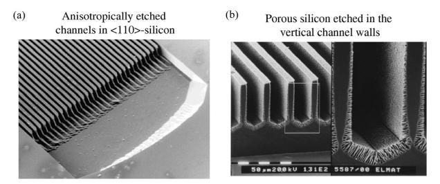
Fig. 1. (a) Overview of the anisotropically etched channel array in the microreactor. (b) Cross-section of the trench type channel arrays in the  $\mu$ IMER with the porous silicon surface layer.
