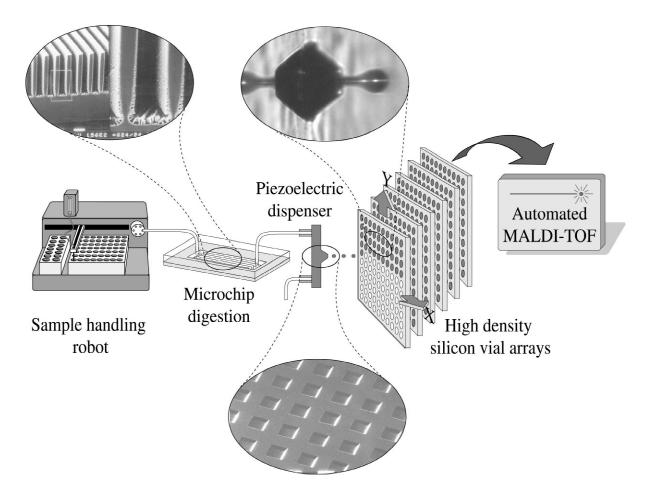
Fig. 8. Schematic drawing of the integrated microanalytical workstation. Inserts show the micromachined parts of the platform.
