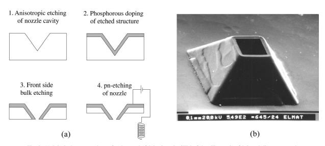
Fig. 2. (a) Principal process scheme for the nozzle fabrication. (b) SEM of the silicon microfabricated dispenser nozzle.
