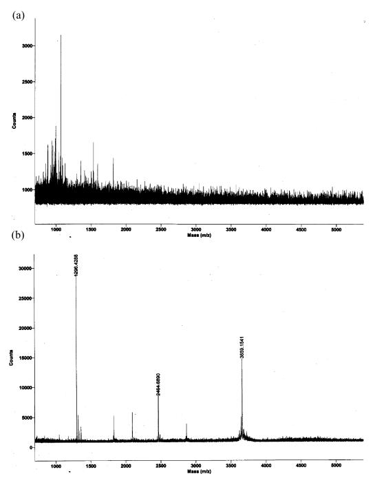
Fig. 6. (a) Mass spectra obtained from ordinary (dried droplet, 50 fmol) sample preparation of a peptide mixture (50 fmol/ $\mu$ l), (b) Mass spectra obtained from 1000 droplets (0.5 fmol) of calibration mixture (50 fmol/ $\mu$ l) deposited in a nanovial.
