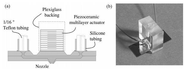
Fig. 3. (a) Schematic drawing of the microdispenser design. (b) Assembled microdevice.
